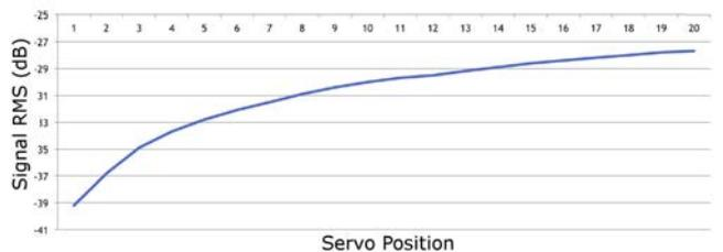
Figure 11 - Effects of velocity control on RMS of signal amplitude
