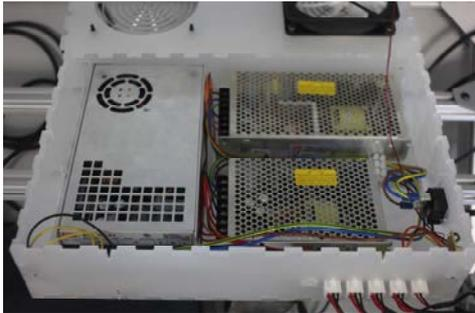
Figure 8 - The power supply module, attached to the aluminium frame of MechBass
