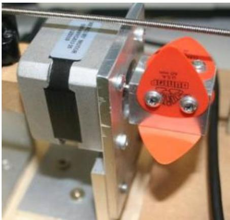
Figure 8 Small Stepper Plucking System
