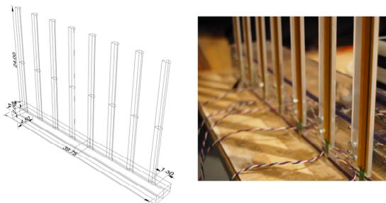
**Figure 4:** The Helio Interface prototype and final rendering, featuring eight upright-mounted membrane potentiometers.
