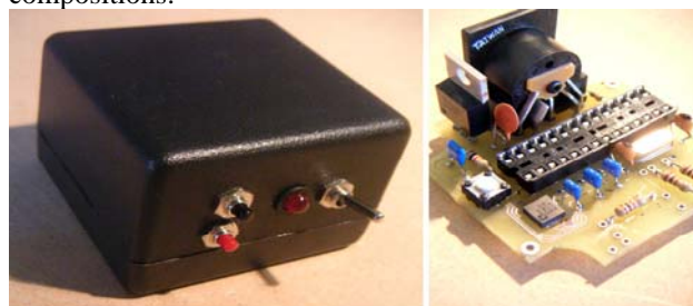
Figure 1 - KiOm encasement and inside circuit board.
